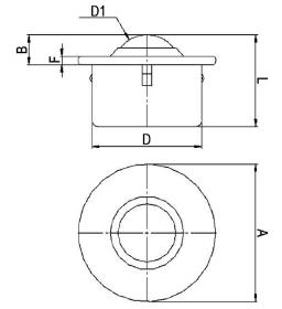
Suggested seating hole size of Ø25mm to Ø25.5mm with a table top material thickness of 2mm.
