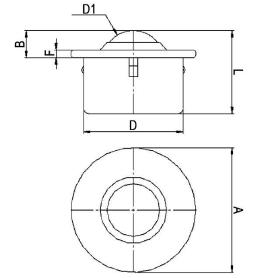
Suggested seating hole size of Ø37mm to Ø37.5mm with a table top material thickness of 3mm.
